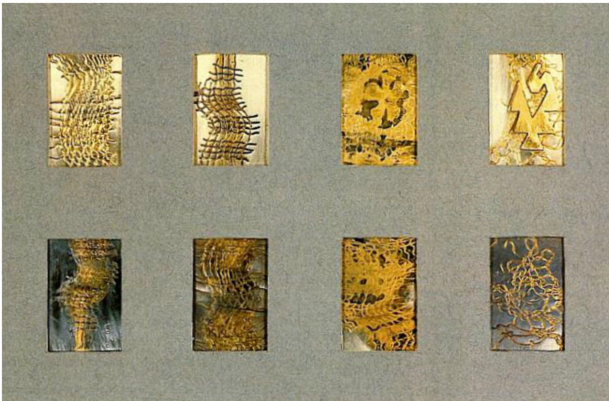
Figure 22. Experimental patina generation of depletion gilded gold plates using 9-carat silver-gold-copper alloy (Del Solar et al. 1982)
